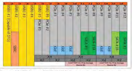
Figure 3-1. HSIO Muxing on SKL PCH U
